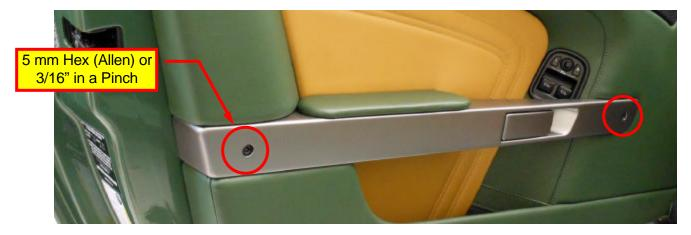
**b)** Grasp the handle using both hands and give it a firm yank (that's me...). If you do not have access to a firm yank, you may find it easier to use a plastic trim tool. Insert your tool (ahem...) between the metal door panel (not the door card) and the rear edge of the handle, and lever [prise] the handle away from the door panel.
