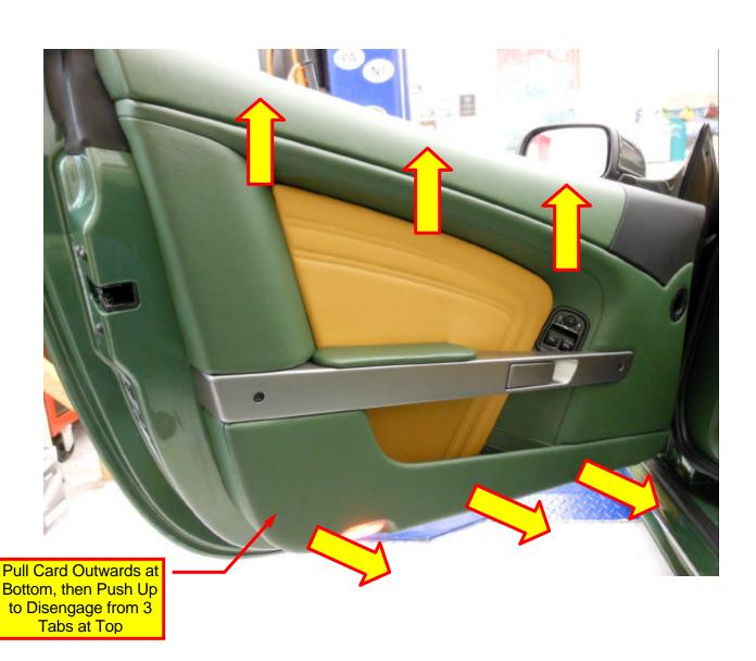
**b)** You will now be left with a door card attached to the door panel by only those 2 pesky connectors. So, while [whilst] balancing the door card with one hand at the back of the card, and the bottom leading edge perched on the tread plate, work the other hand into the gap between the card and the door bottom and disconnect those connectors.
