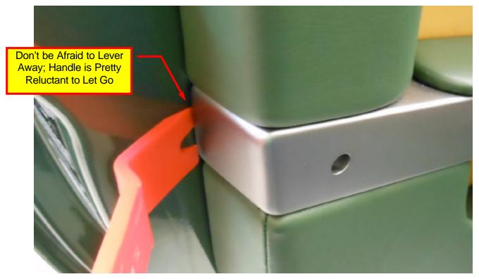
**c)** Once you've managed to loosen the door handle, you can work both ends until it is completely free of the door panel. Do not pull the handle away from the door too far since the door latch mechanism cable is still attached to the door handle (**see next step first**).
