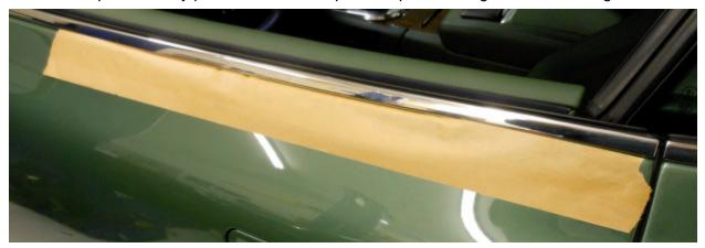
**c)** Using an automotive plastic trim removal tool, gently pry up [*prise*] the chrome strip, starting at the back edge of the door, and gradually work your way forward. Once you've pried [*prised*] at least half way down the length, you can just pull up the rest by hand without using the tool.
