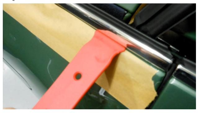
**d)** When re-installing the strip, begin at the front edge, using a rubber mallet or the heel of your hand to firmly tap the trim into place. Once fully installed, tap over the whole length to assure that it is firmly in place.
