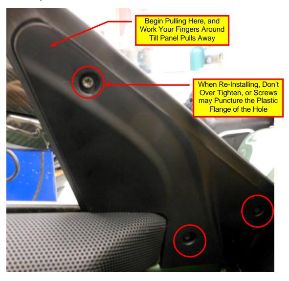
**c)** This is rather flimsy plastic, so when re-installing, do not over tighten the screws otherwise they may punch through the recessed hole flange (don't ask...).
