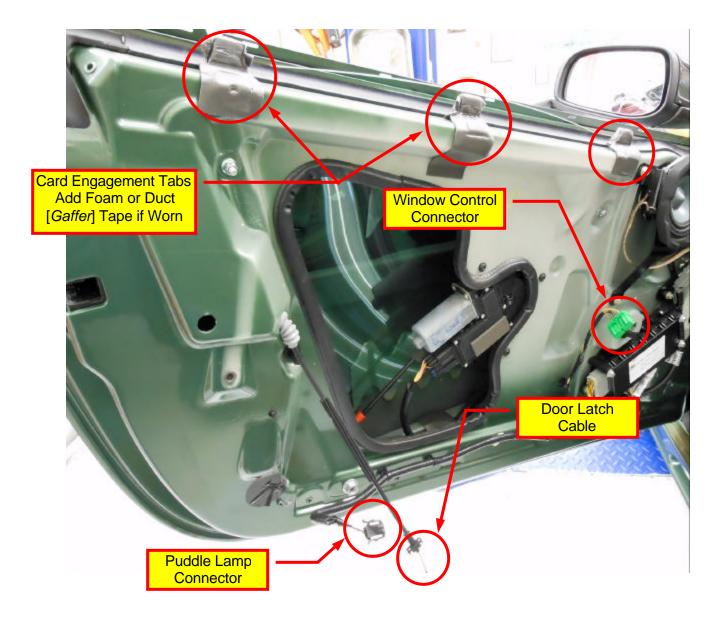
**c)** Remove card and place on a cloth-protected firm working surface with the facing side down.
