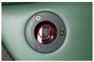
**c)** Remove the leather trim panel at the back of the door cap (held only by sticky tape or velcro) to access the last door card Torx screw (T15). The bracket removes with the screw.
